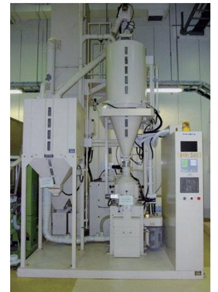
Figure 2.2 Rice milling machine
