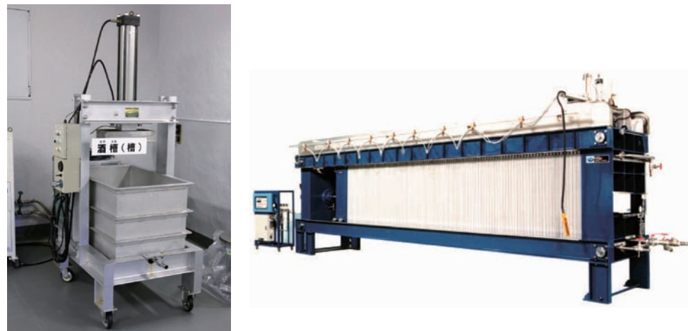
Figure 2.8 Mash filtration machines
